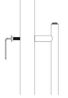
**3.** Present the pull handle up to the bolts and tighten. Ensure the plastic washer is in the correct position.
