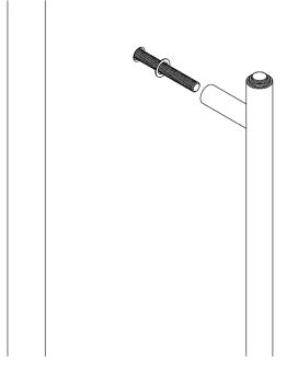
**2.** Fit the bolts through the fixing holes and place the washer on the door side where the pull handle will be fitted.
