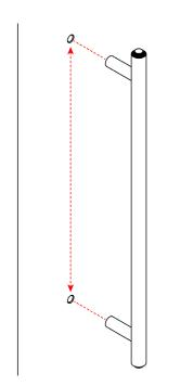
**1.** Drill holes to the appropriate size, in the position required and counter sink.
