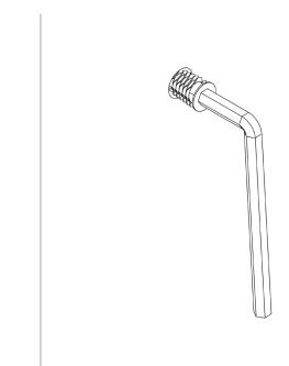
**2.** Push the wood screws into the newly drilled holes, and tighten with allen key until flush.
