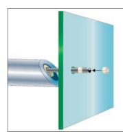
Fixing to glass doors uses the same methods as above but when fixing please use the white plastic sleeve in the bolt hole to protect the glass.
