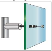
Use the same method ad above but please use the white plastic washers and the white plastic or black rubber sleeves to protect the glass inside the drilled hole.
